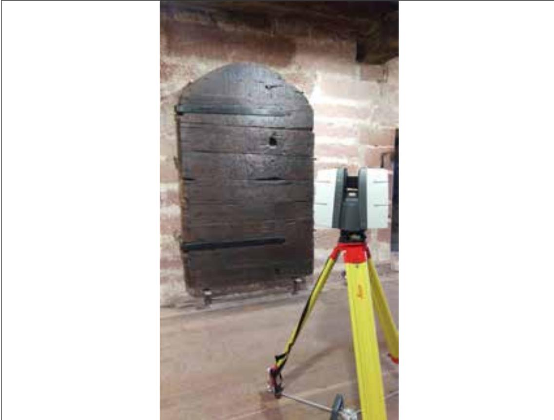
Figure 6: Leica P40 laser scanner set up to scan the medieval door.
