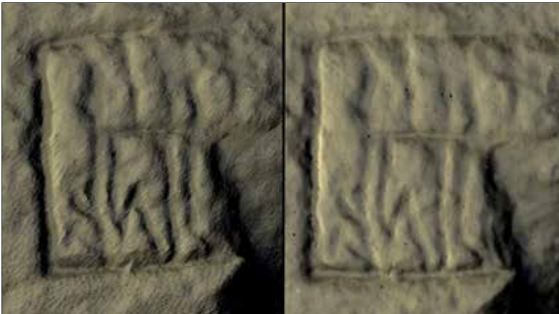
Figure 5: Virtual raking light from the left side of both PTM images. Left: PTM image from laser scan data. Right: PTM image from SfM photogrammetry. Note how the depths of the shadows are greater from the laser scan data, and the better clarity of several of the lower line of runes, although striping features across the surface. The symbol on the bottom left looks substantially different between the datasets.
