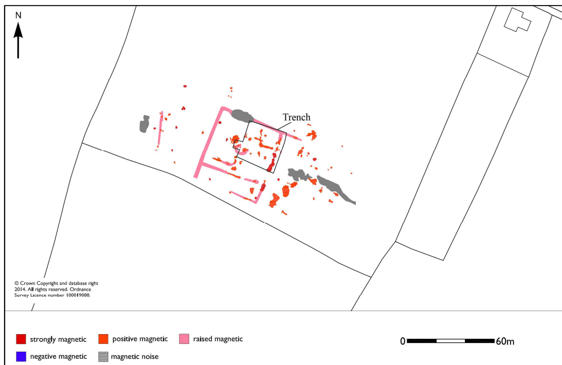
Fig 33: Graphical summary of significant caesium magnetometer anomalies at Kellaways and location of excavation trench (© Historic England)
