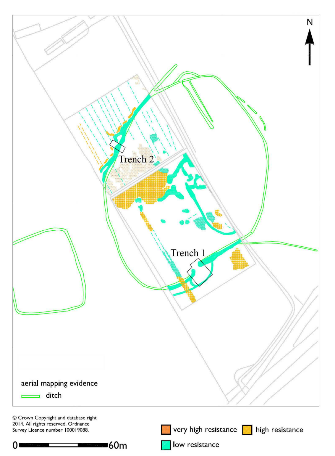
Fig 19: Graphical summary of significant earth resistance anomalies at the southern enclosure at Paxcroft and location of excavation trenches (adapted from Linford et al 2015a)
