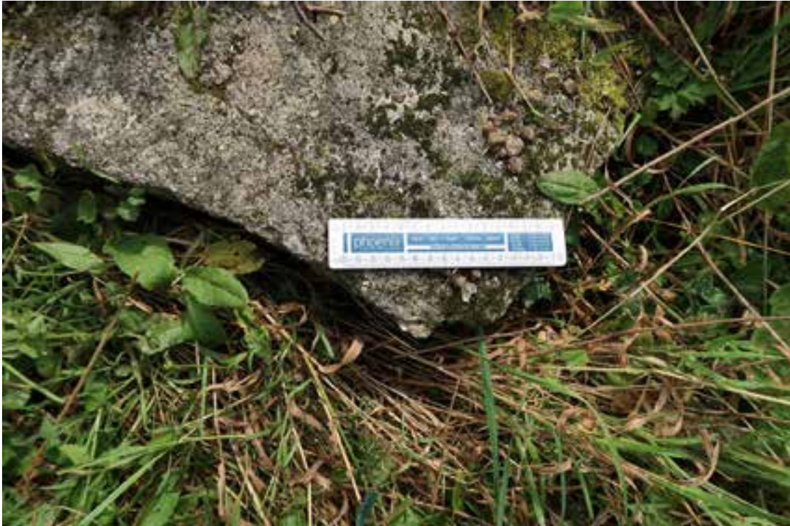
Figure 36. Granite block with traces of a drilled charge hole from rubble spread – 15cm scale (© Historic England, photograph Olaf Bayer).
