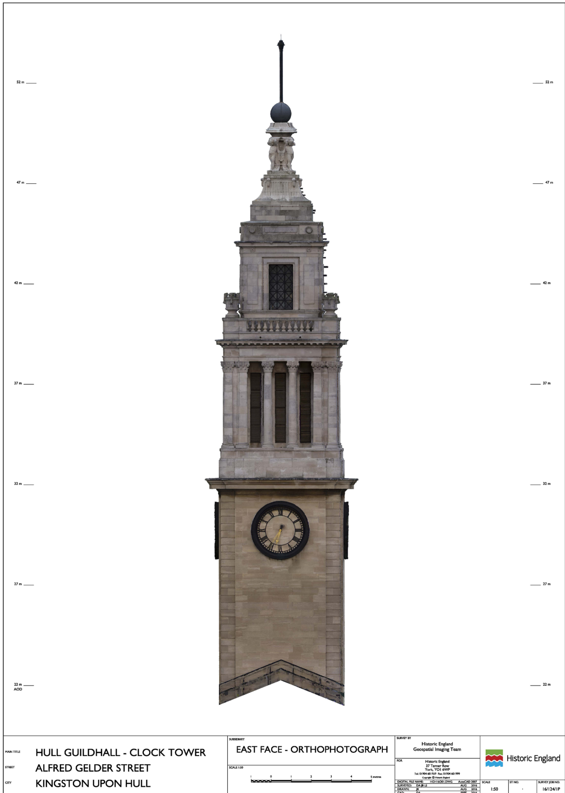
Fig. 20: Orthophotograph of the Lowgate elevation of the clock tower, with time ball, as constructed. © Historic England
