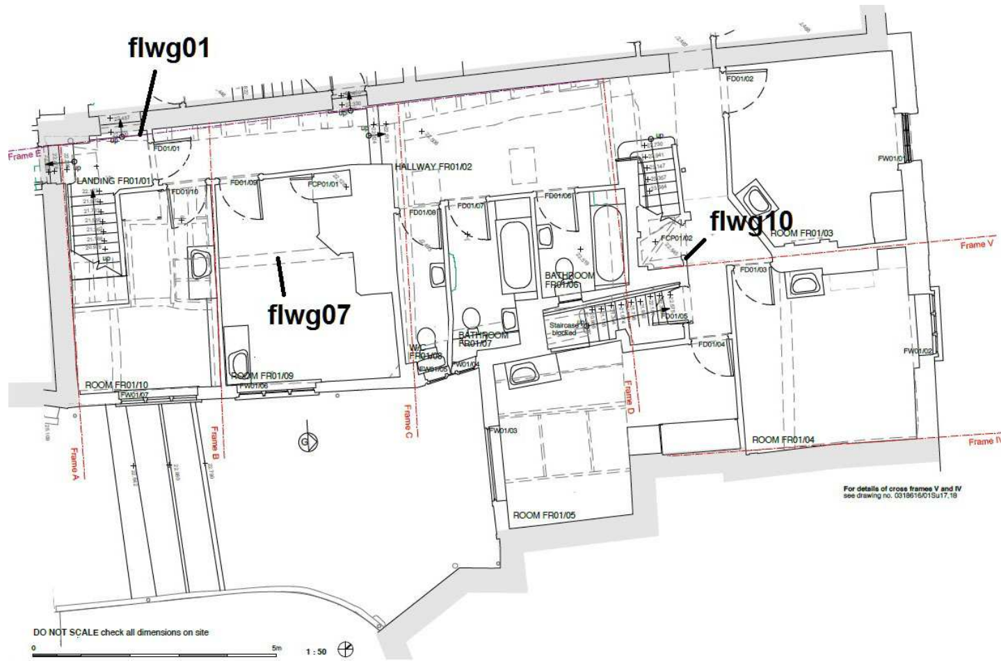
Figure 17: Plan of the Westgate range showing the locations of some of the sampled timbers (after Butler Hegarty Architects)
