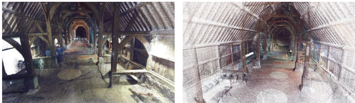
Figure 11-18 3D view of 20 minute REVO (left) and 2 minute REVO (right)
