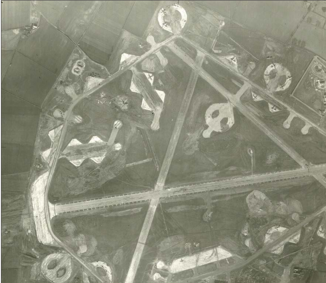
Figure 2: RAF Upper Heyford, this view shows the flying field shortly after its modification to accept SAC bombers. New features include an extended runway and additional aircraft parking areas. (c) Historic England 540/673/12Feb1952/frame 4272.
