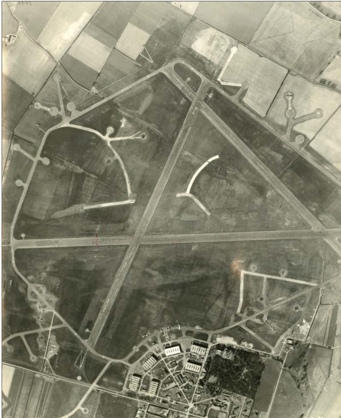
Figure 1: RAF Upper Heyford, during the war the most significant alterations to the flying field included the laying of concrete runways and taxiways. (c) Historic England CPE/UK2013/16Apr47
