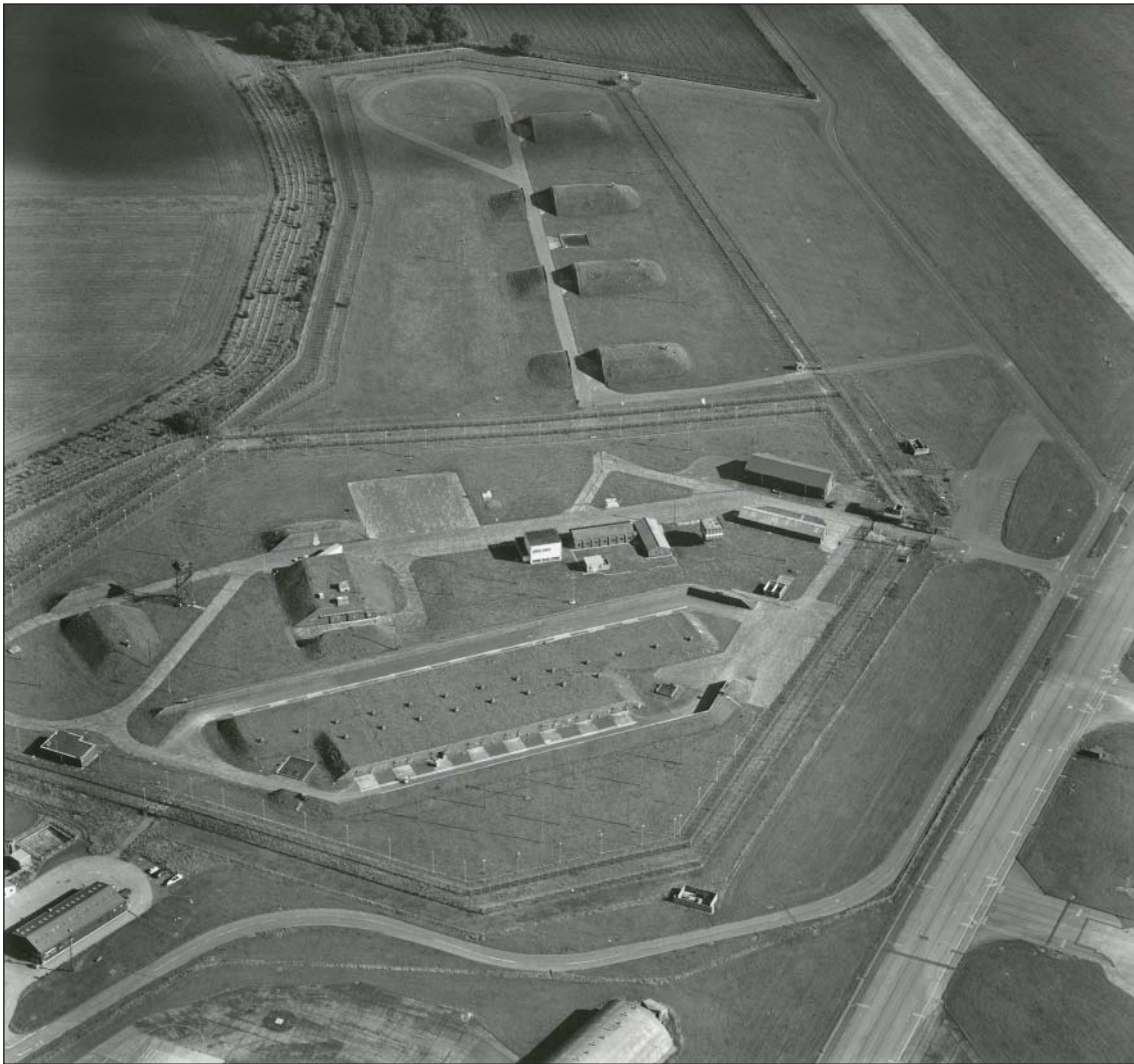
Figure 9: RAF Upper Heyford, Northern Bombs Stores in 1999, showing the second phase with a new storage building and a reduced defended perimeter. (c) Historic England 18537/09
