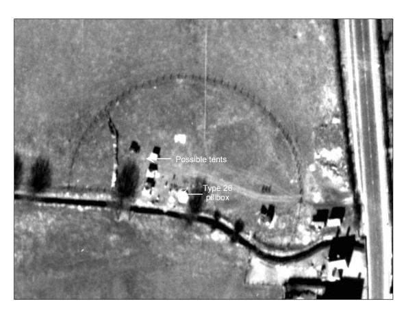
Figure 37. A previously unrecorded pillbox, type FW3/26 at Longford (NRHE: 1583785), with nearby tents and a fenced off perimeter. NMR RAF/106G/UK/1293 RV 6023 25-MAR-1946 Historic England RAF Photography
