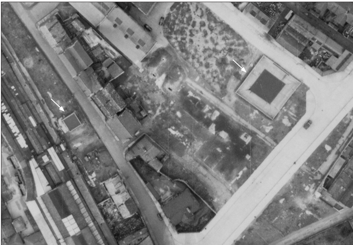
Fig 19: Emergency Water Supplies on Outram Street (right) and Church Street (left), indicated by arrows. Two covered trench shelters are also located just above the centre of the image RAF/106G/UK/873 RV 6181 01-OCT-1945 Historic England Archive RAF Photography (detail).
