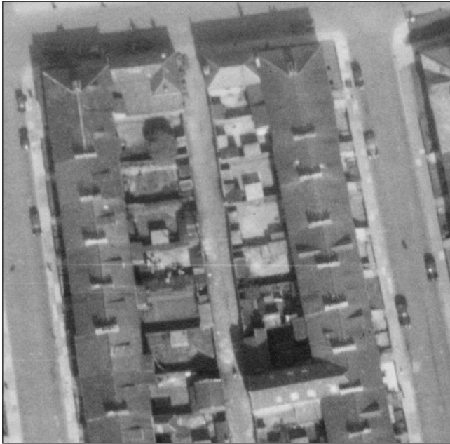
Fig 15: Domestic surface shelters in the back yards of houses on Foyle Street and Frederick Street. The shelters are the small, flat-roofed rectangular structures abutting the walls of the back yards. RAF/106G/UK/745 RV 6240 28-AUG-1945 Historic England Archive RAF Photography (detail).
