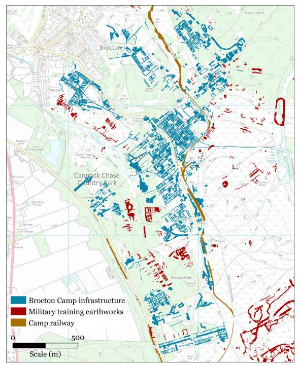
Fig 51: The remains of Brocton Camp include hut foundations, drains and roads (highlighted in blue). These are surrounded by extensive training earthworks (in red). A' to 'T' refer to the camp lines, as denoted on the 1916 plan. Archaeological map © Historic England; Base map © Crown Copyright and database right 2018. All rights reserved. Ordnance Survey Licence number 100019088.
