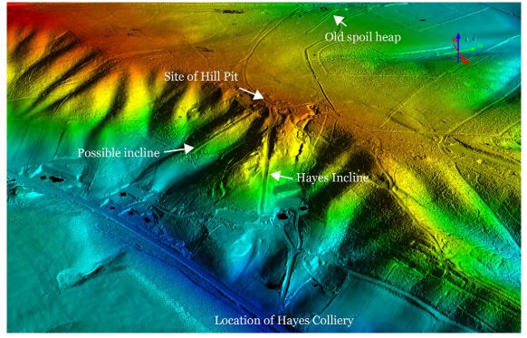
Fig 85: Lidar showing Hayes incline and the earthworks of a second possible incline on the left. Lidar DTM 04-MAY-2016 © Historic England; source Staffordshire County Council/Fugro BV Geospatial.
