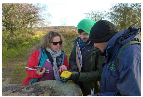
Fig 18: Comparing mobile recording devices with a handheld mapping-grade GNSS receiver out on the Chase, November 2016 © Historic England.
