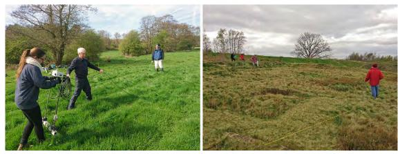
Fig 13: Volunteers using a resistivity meter at Sheepwash Farm (left) and carrying out magnetometry survey over the medieval building platform within Castle Ring hillfort (right), April 2017 © Historic England.
