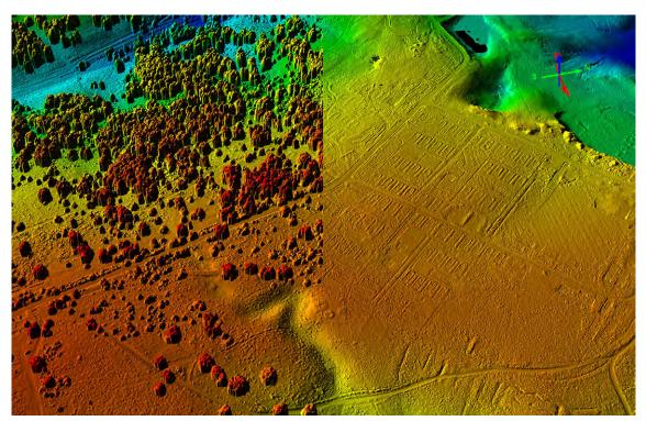
Fig 43: Brocton Camp is mostly covered by scrub woodland, reducing the visibility of the archaeology. This lidar image depicts the surface model on the left, and terrain model on the right, where the vegetation has been stripped away. Lidar DSM and DTM 04-MAY-2016 © Historic England; source Staffordshire County Council/Fugro BV Geospatial.
