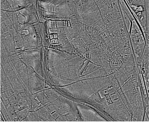
Fig 21: Brocton Camp: Simple Local Relief Model (LRM) lidar. Although more difficult to interpret on the whole, visualisations such as this display shallow cut features with more clarity. Lidar DTM 04-MAY-2016 © Historic England; source Staffordshire County Council/Fugro BV Geospatial.
