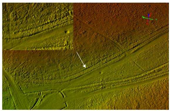
Fig 54: The indentations of the railway sleepers still survive as earthworks. Lidar DTM 04-MAY-2016 © Historic England; source Staffordshire County Council/Fugro BV Geospatial.
