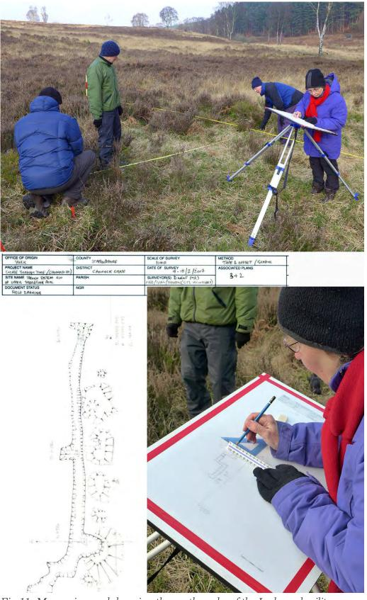
Fig 11: Measuring and drawing the earthworks of the L-shaped military practice trench near Uppersherbrook Pool, February 2017 c Historic England.
