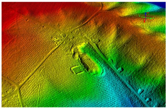
Fig 36: The spoil heap to Fairoak Colliery Pit Number 2. The remains are now surrounded by dense forestry plantation but the lidar visualisation reveals the extent of the site. Lidar DTM 04-MAY-2016 © Historic England; source Staffordshire County Council/Fugro BV Geospatial.
