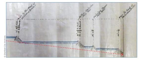
**Plate 4:** Extract from a plan showing the arrangement of weirs between Hillsborough Bridge and Owlerton Bridge illustrating how weirs could be used to artificially control the level of water within the river.
