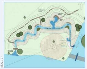
Plate 45: ARUPs Plan for Rodley Weir bypass channel
