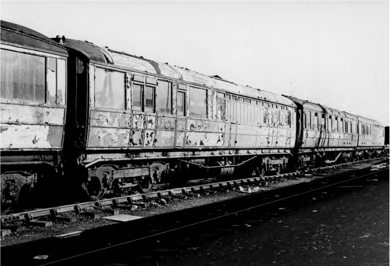
Plate 47: The derelict condition of four of the Carstairs stabled mobile control rooms Note the fuel tank under SC16198E which is the generator coach.
