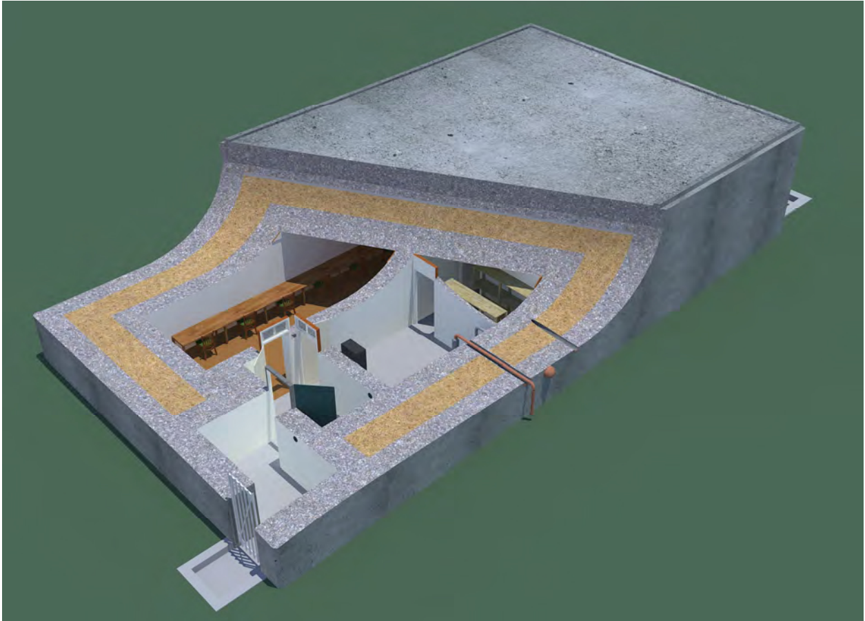
Fig 15: Exploded view of Chester District Type A2 Control Room Computer-generated model. Paul Bellamy
