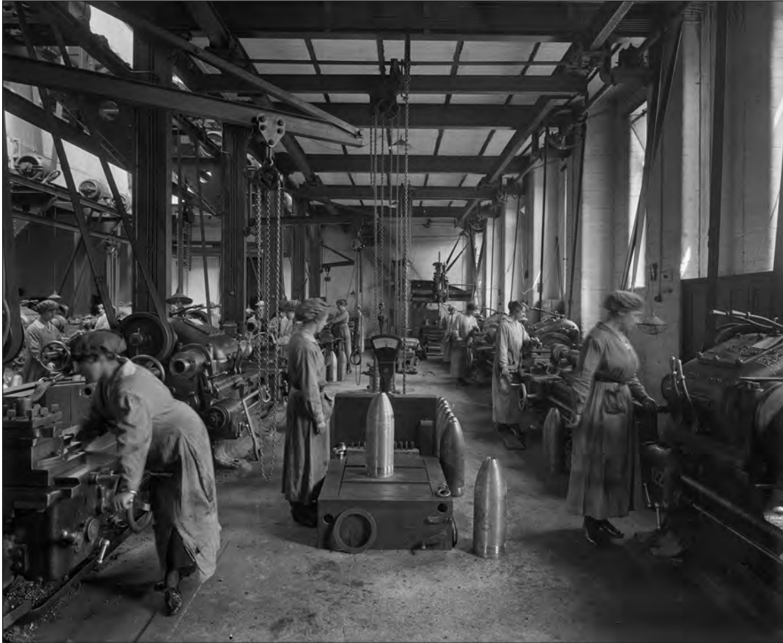
Fig. 4.13. NSF Liverpool (Cunard), women workers in Rimrose Road turning large calibre (8-inch) shells 1917 (© Historic England BL/24001/09).
