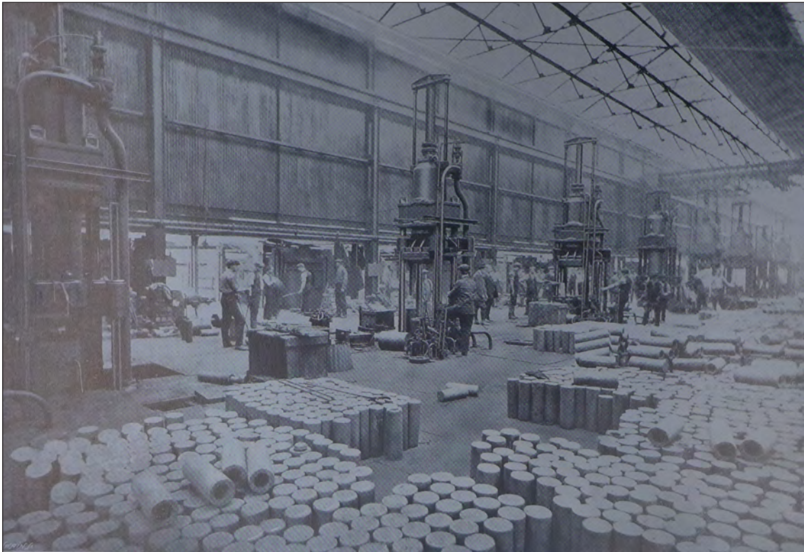
Fig. 4.14 NPF Sheffield (Tinsley), shell forge at work, 1916. The furnaces can be seen to the rear left, with presses in the foreground. Both steel billets and finished shell blanks are stacked nearby (TNA MUN5/157).
