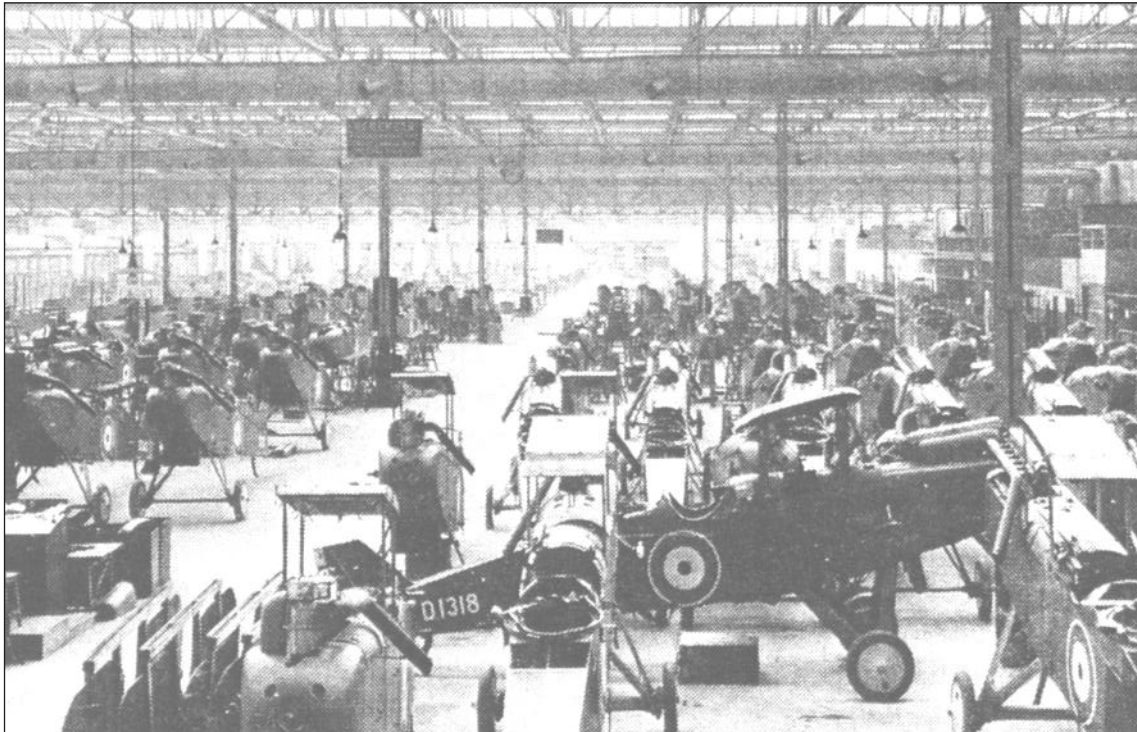
Fig. 4.38. NAF No.2 Heaton Chapel interior in 1918, showing DH9 aircraft under assembly ( http://en.wikipedia.org/wiki/National_Aircraft_Factory_No._2 #mediaviewer/File:NAF_No.2_1918.jpg, accessed 04/11/2014).
