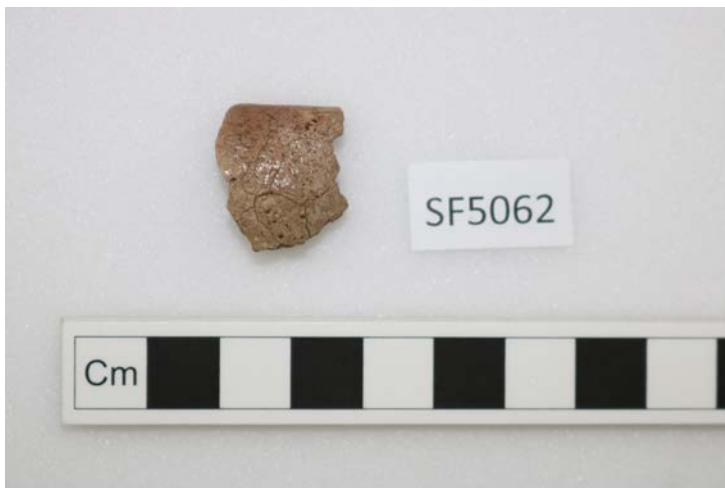
Fig 4. (551) SF 5062. The outside of the crucible fragment has a bright, shiny, glaze-like surface. This vitrification usually occurs when technical ceramics come into contact with fluxes like fuel ash.
