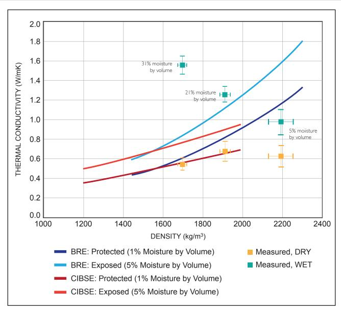
*Figure 7*: Comparison of measured values with design values from BRE Digest 108 and CIBSE Guide A. Both the Digest and the Guide assume moisture contents of 1% and 5% by volume for protected and exposed brickwork, respectively. The measured wet thermal conductivities range between 5% and 31% by volume.
