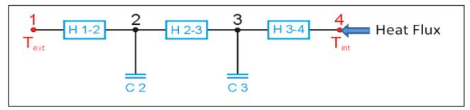
Figure A8: Example of a wall modelled as a network of conductances and capacitances
