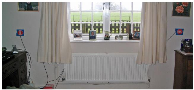
Figure A2: Typical heat flux sensor and room temperature measurement locations.
