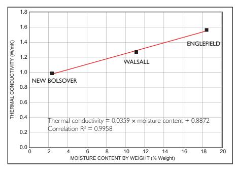
Although the graph in *Figure 3* suggests that there is a linear relationship between the capillarysaturation moisture content by weight and the thermal conductivity, this may be fortuitous: it may not be the case that all bricks fit this relationship.
