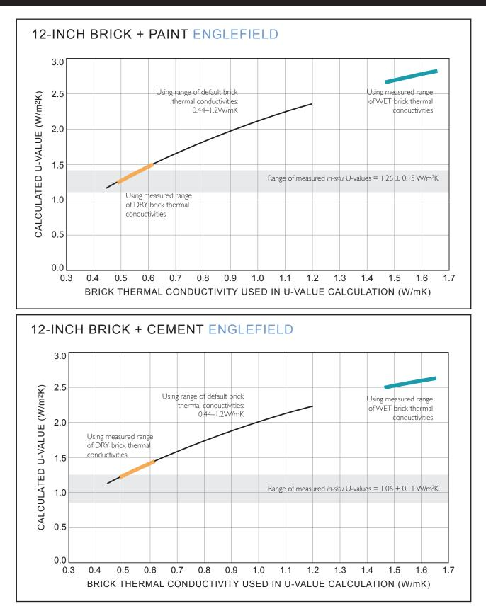
*Figure 4b*: Comparison of measured U-values with calculated values using the BuildDesk software with measured dry and wet brick thermal conductivities of the Englefield brick sample.
