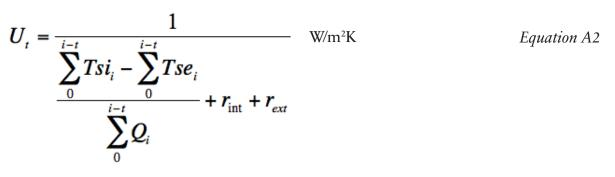
where *Tsi* and *Tse* are the internal and external surface temperatures respectively.
