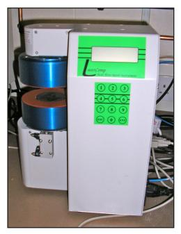
*Figure 1*: Lasercomp Fox 50 thermal conductivity apparatus
