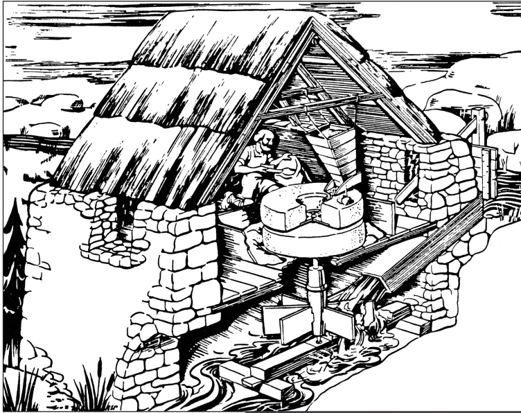
Figure 1 – A reconstruction drawing of a horizontal mill based on an example from the Shetlands, Scotland (from John Storck and Walter Dorwin Teague, Flour for Man's Bread: A History of Milling , illustrated by Harold Rydell (University of Minnesota Press, 1952). Copyright 1952 by the University of Minnesota, renewed 1980)
