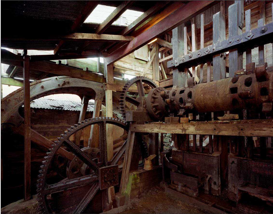
Figure 4 – The stamps and waterwheel at Tolgus tin streaming works, near Redruth, Cornwall (Peter Williams © Crown Copyright. Historic England bb98_13519)
