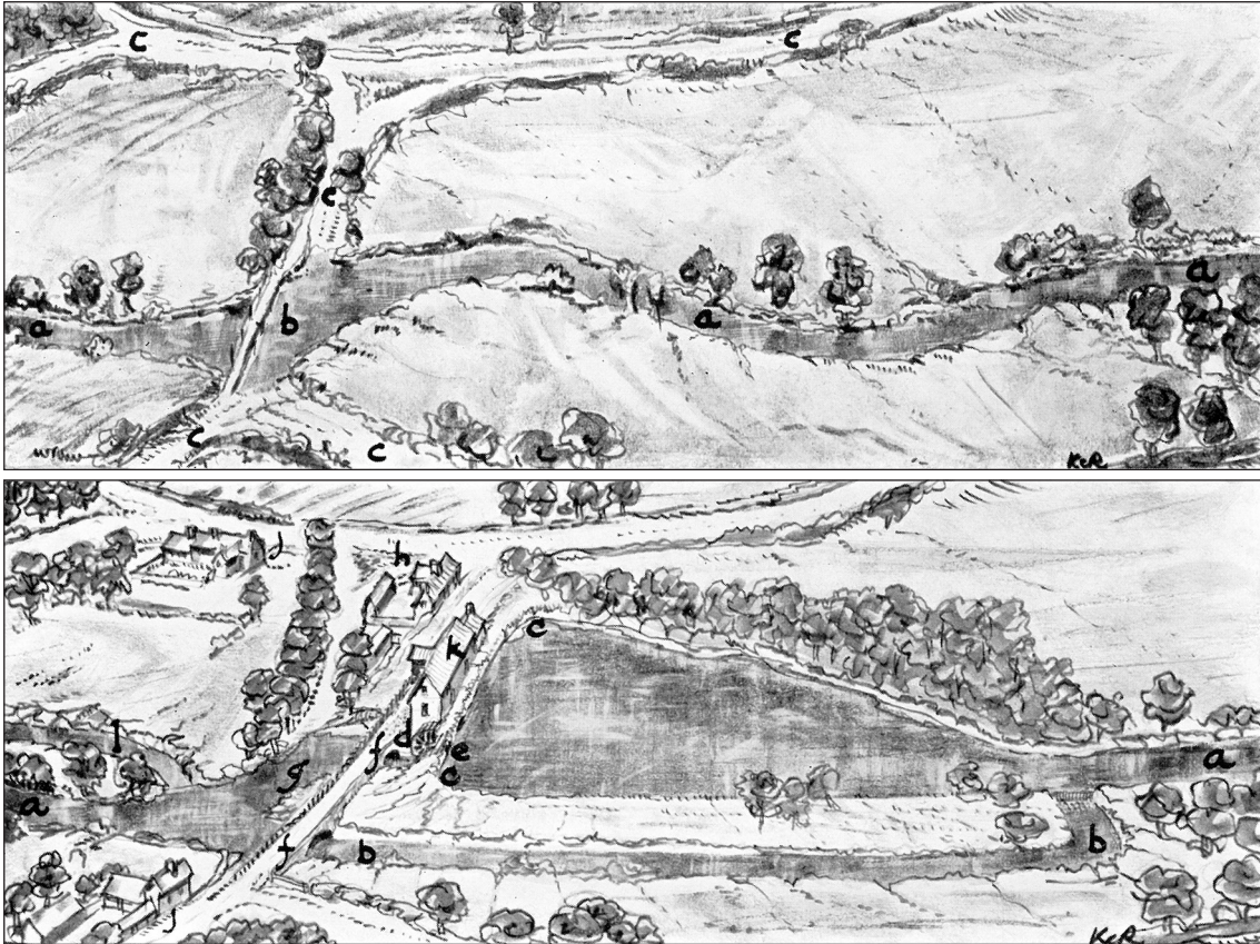
Figure 9 – Two sketches showing the changes on a length of river resulting from the building of a watermill, in this case a mill on the natural channel with a bypass leat. Before (above); a = river, b = ford with footbridge, c = lanes: and after (below); a = river, b = overflow leat, c = dam, d-e = spillway with sluice, f = road bridge, g = old ford, h = mill farm, j = cottages, k = watermill, l = leat taking water from the river to supply a mill further downstream (Reid 1959, Plate 2; Plate 3, © SPAB Mills Section, with permission)
