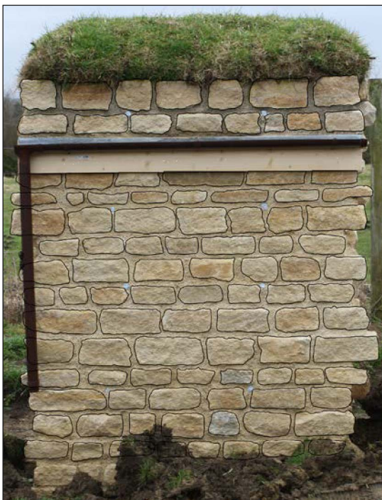
Figure 3.14 Location of points for Protimeter surveys, July 2009 to January 2012 on wall 1 as an example of the method used on both sides of each wall. ©Heather Viles, University of Oxford
