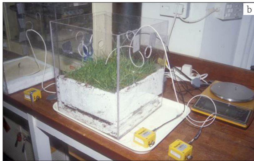
Figure 1.13a, b Experimental set-up with stone and soft capping in Perspex boxes. (a Iain McCaig © Historic England, b Chris Wood © Historic England)
