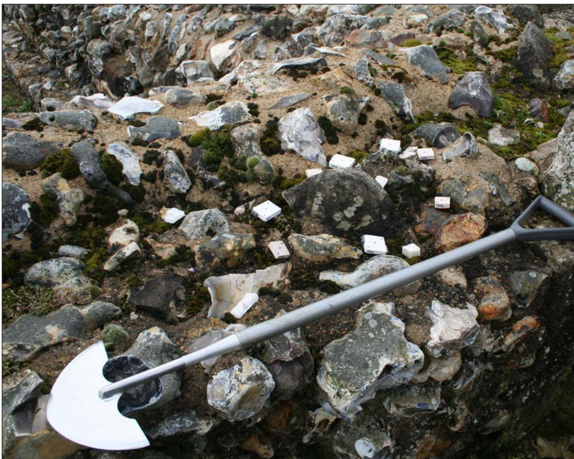
Figure 3.20 Gypsum and limestone blocks and calcite crystals on test strip 3, before covering with the sedum soft capping. ©Heather Viles, University of Oxford
