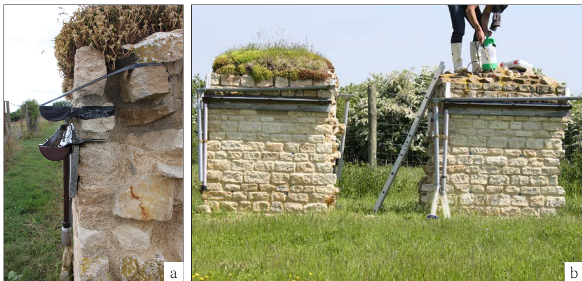
Figure 3.17 (a) Layout of the two-gutter system to collect runoff and shed water separately (b) spraying in action on the cement hard cap. ©Heather Viles, University of Oxford
