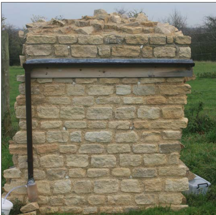
Figure 3.15 Guttering with lead flashing to collect runoff. ©Heather Viles, University of Oxford
