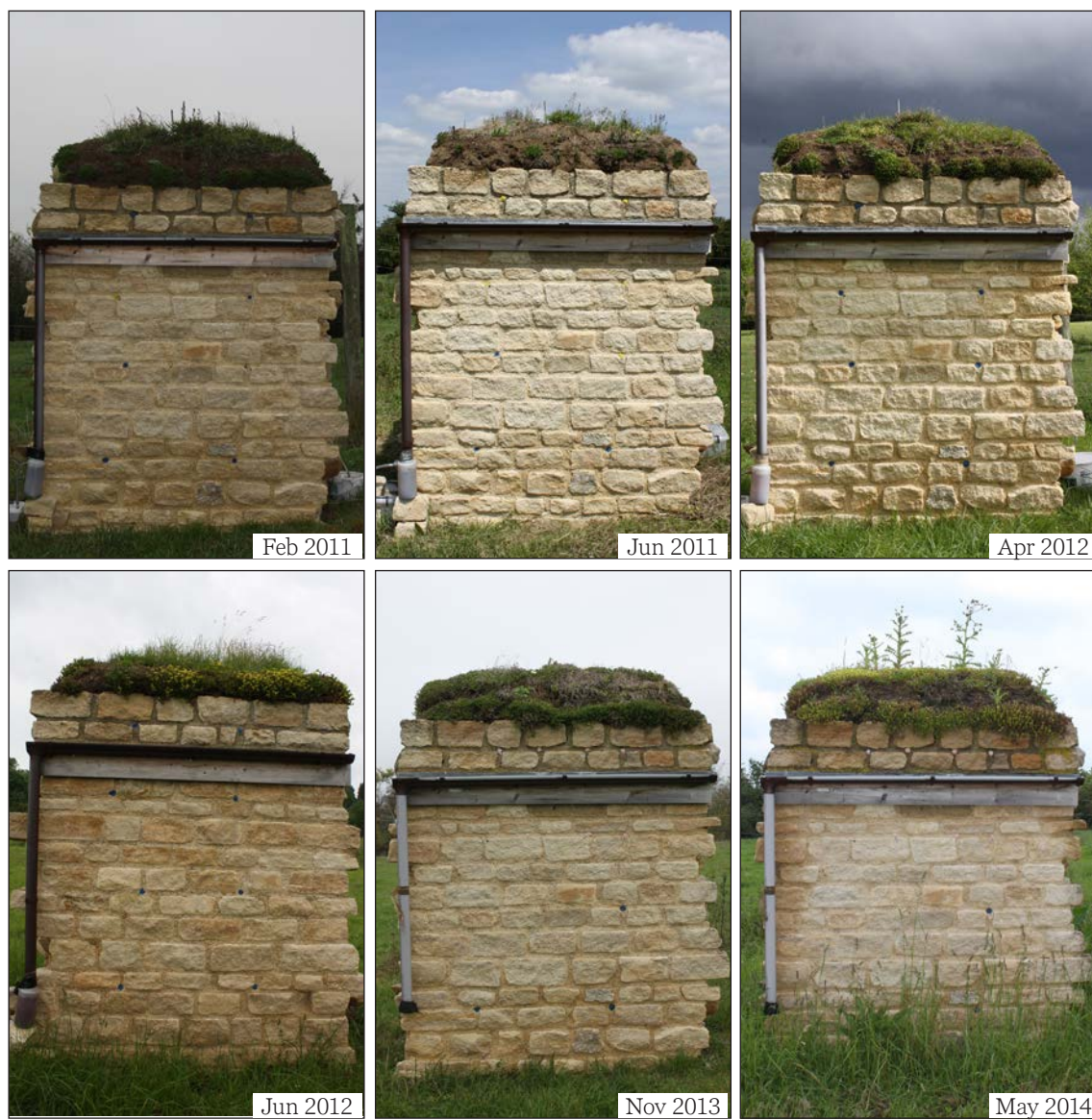
Figure 4.34 Changing appearance of soft capping on the Wytham Woods test walls. ©Heather Viles, University of Oxford
