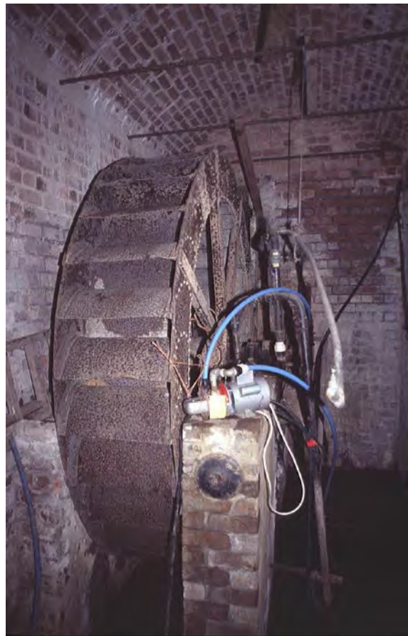
Fig. 15. Burton Court Pump-house, Eardisland: waterwheel and pump, with their successor!
