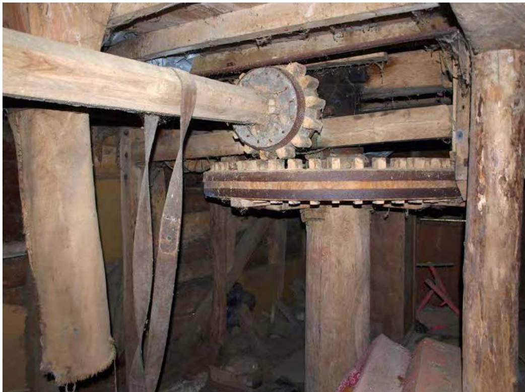
Fig. 21. Wegnall Mill, Rodd Nash & Little Brampton: 18 th cent. machinery on the stone floor.
