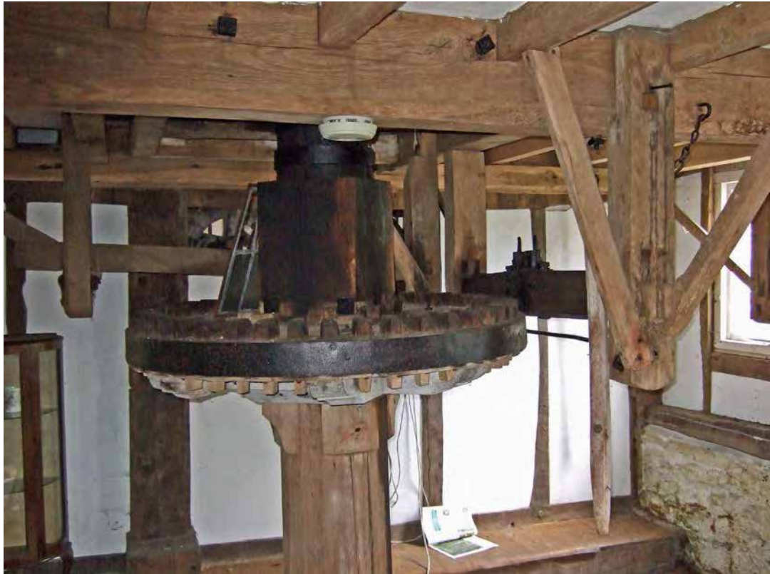
Fig. 26. Burton Mill, Eardisland: 18 th century crownwheel & upright shaft.
