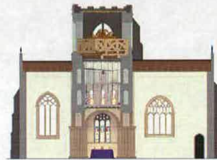
Figure 11 St Mary's, Attleborough, Norfolk Section through tower and transepts looking east Period F As existing
