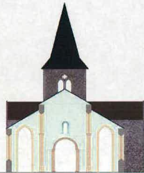
Figure 6 St Mary's, Attleborough, Norfolk Section through nave looking east Period C c.1400
