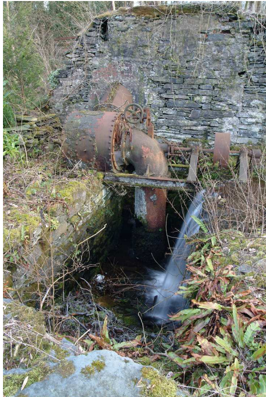
Fig 102. Gilkes turbine no. 2065 at the sawmill. (NMR DP003446)
