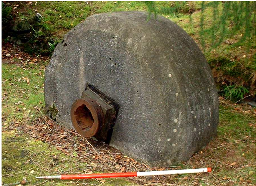
Figure 33. Edge-runner MS26 and axle mount, photographed in 2001
