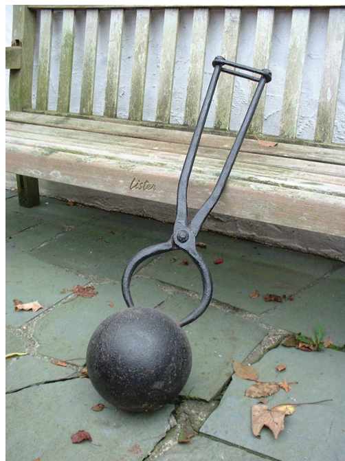
Figure 72. The mortar ball and carrying callipers used for test firings on the proofing range
