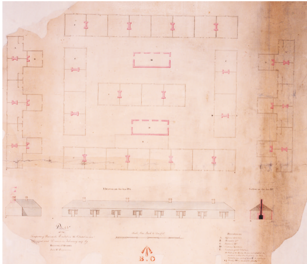
Figure 50 Plan of the Napoleonic Temporary Barracks in the Citadel, dated 1817. The large reectangular arrangement comprised the soldiers barracks and cooking kitchens, with separate officers' blocks on the east and west sides (north is at the top)(extract of MPH/1/506 © The Public Record Office)
