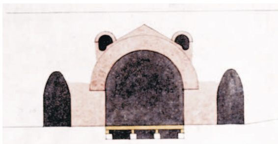
Figure 38 Clarence Tower; north-south section of the main magazine, showing the semi-circular vault, suspended timber floor and parabolic vaults of the lighting passage (PRO: Work/31/309 (extract) © The Public Record Office, by kind permission)
