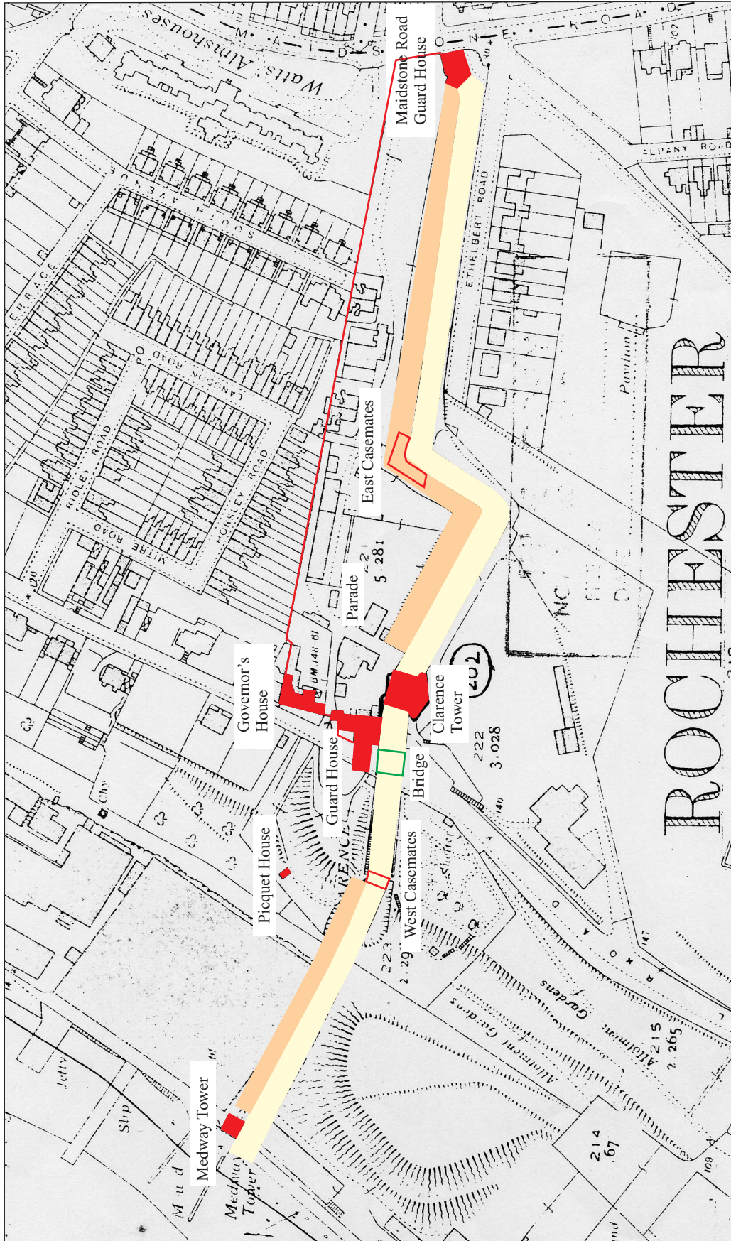
Figure 3 Plan showing the principal elements of the defences built at Fort Clarence, 1808-15. Sand = rampart; yellow = ditch; solid red = building above ground; outline red = building below ground; green = bridge across the Borstal to Rochester road (Reproduced by permission of the Director General of the Ordnance Survey)
