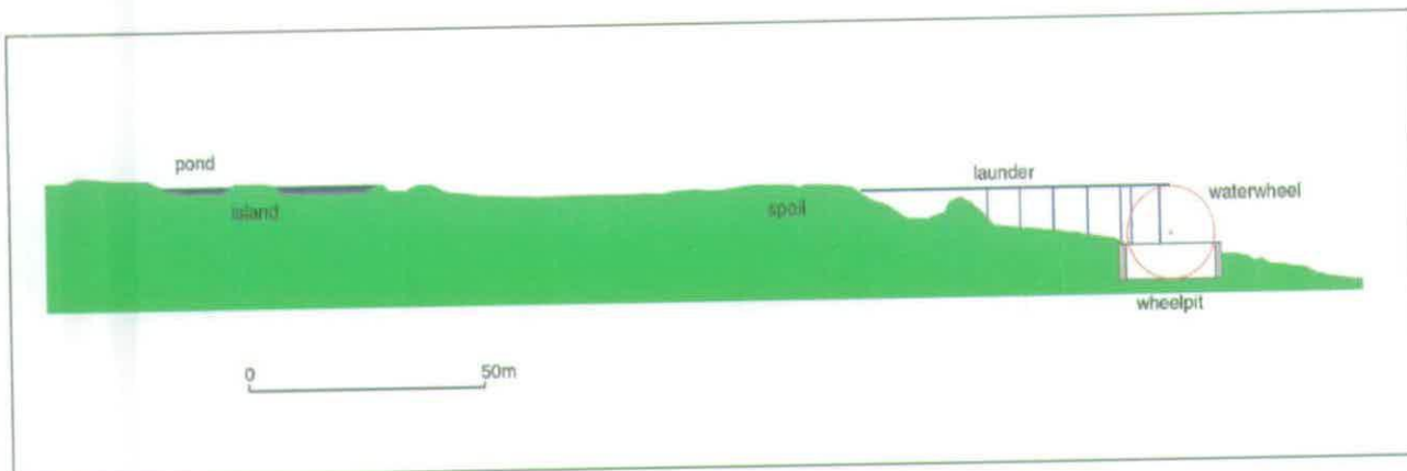
Fig. 5. Composite section showing relative heights of the pond, spoil heap and waterwheel.
