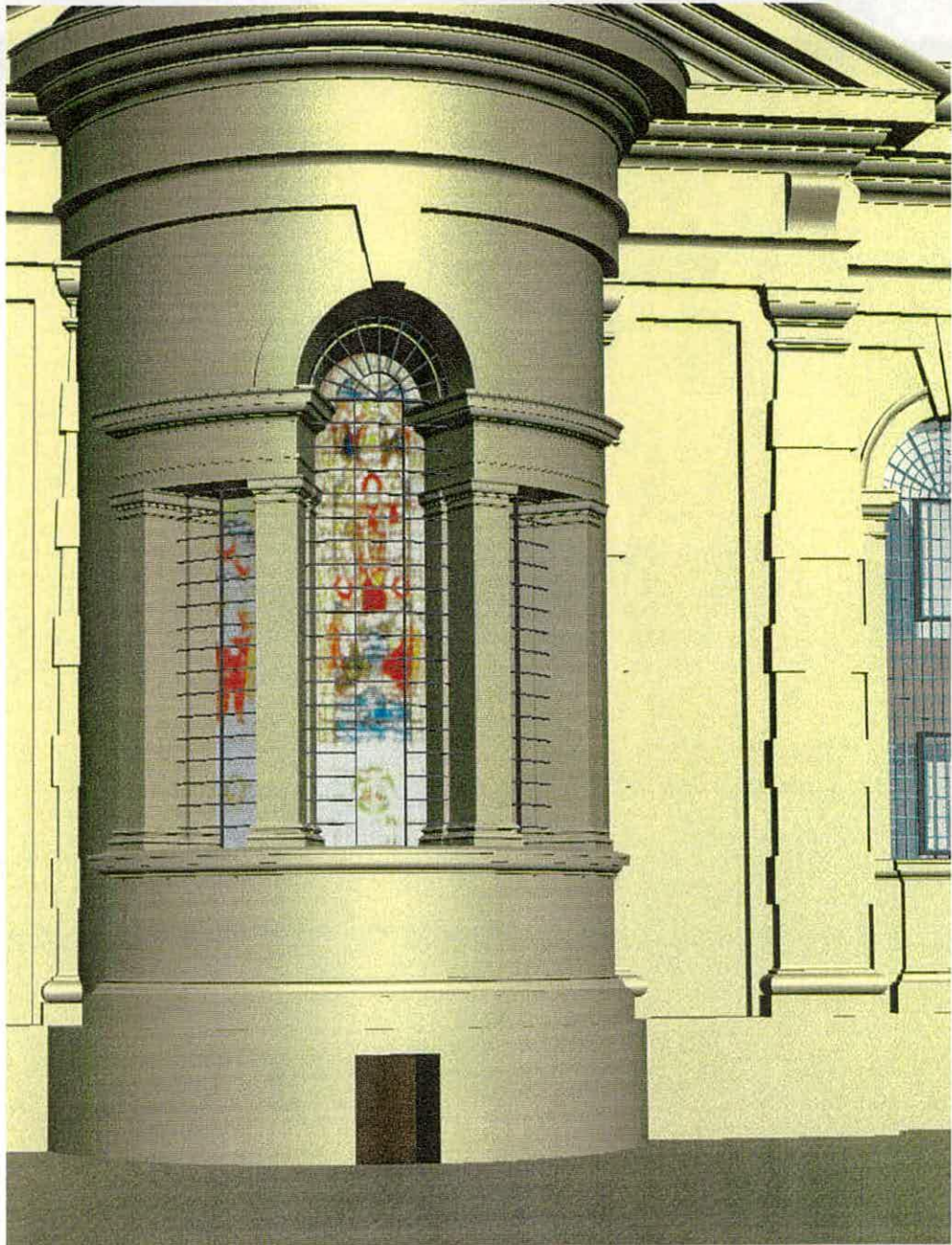
Fig. 33, a perspective reconstruction the Powell east window of 1913, installed behind the original ferramenta, close to the face of the inner wall.
