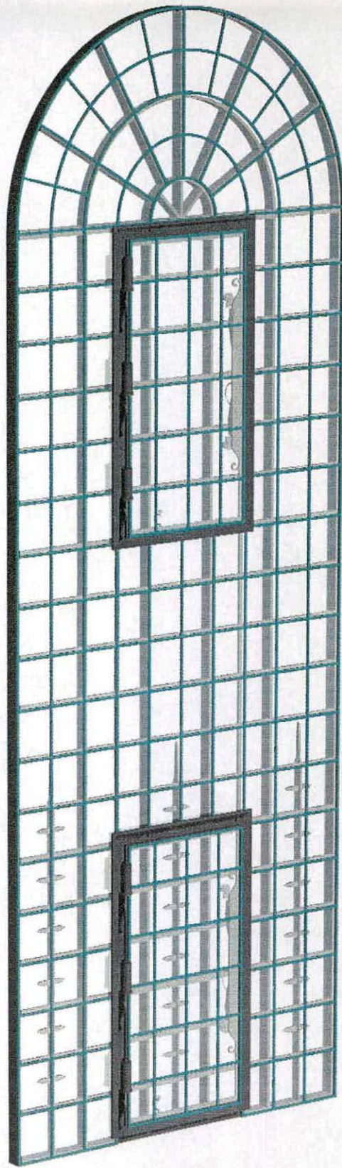
Fig. 20, a reconstruction drawing of a standard window showing how the pattern of the glazing is designed to fit with the ferramenta
