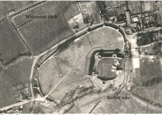
Fig 48: Extract of RAF vertical showing traces of barbed wire entanglements around the south-east corner of the castle and widened ditches to the north, to impede access from low-lying ground. Note the presence of the pound on the outside of the walls RAF/HLA/430/RV 6044 26-MAR-1942 Historic England RAF Photography
