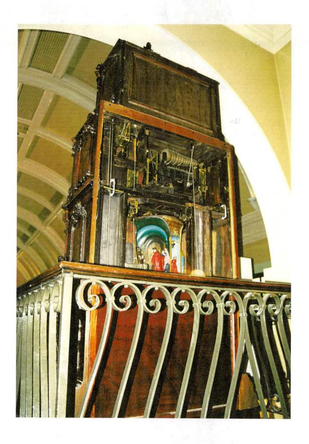
Figure 15; Photograph of the Apostle Clock, from the north staircase, showing the clear panel inserted into the back face of the clock to allow the viewing of the internal mechanisms
