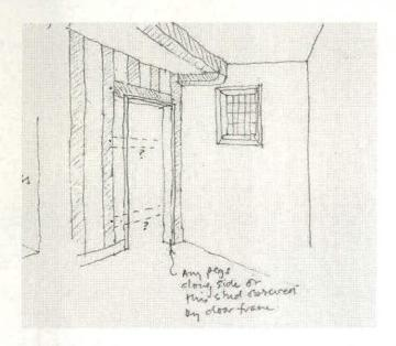
Figure 18 North wing. First floor. Sketch showing the position of the sixteenth century window opening (now blocked) which lit the former staircase bay at the northern (service) end of the house
