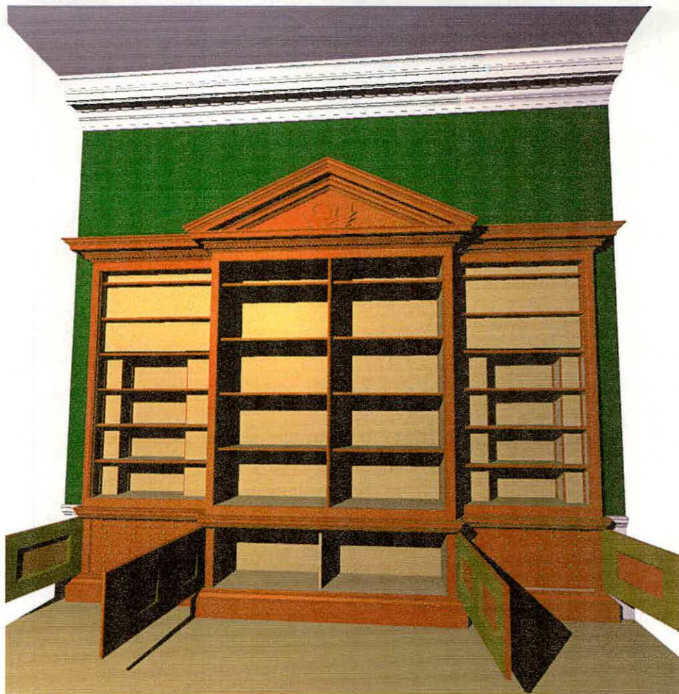
Figure 34, a perspective view showing how the bookcases on the south wall would appear with the cupboard doors open if restored according to our preferred options.
