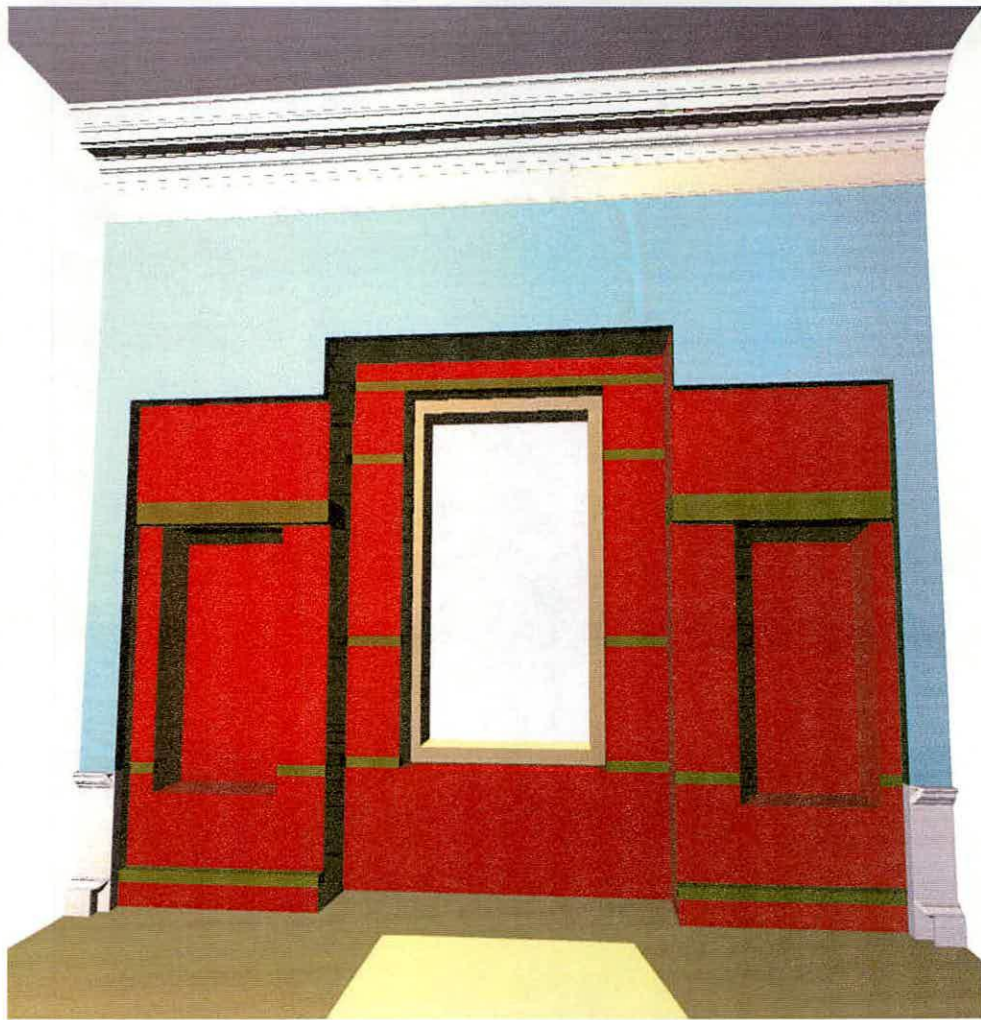
Figure 30, a reconstruction of the north wall, showing it altered by the removal of brick to receive the modified bookcases, as it might have appeared c 1863.
