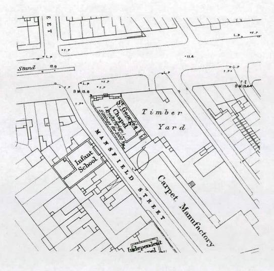
Fig. 16 Detail of 1875 edition of the 5 feet to 1 mile Ordnance Survey map of the Southwark area, showing an enlargement of St George's chapel. The positions of the gallery and its supports are shown, together with the caption 'Sittings for 1000'.
