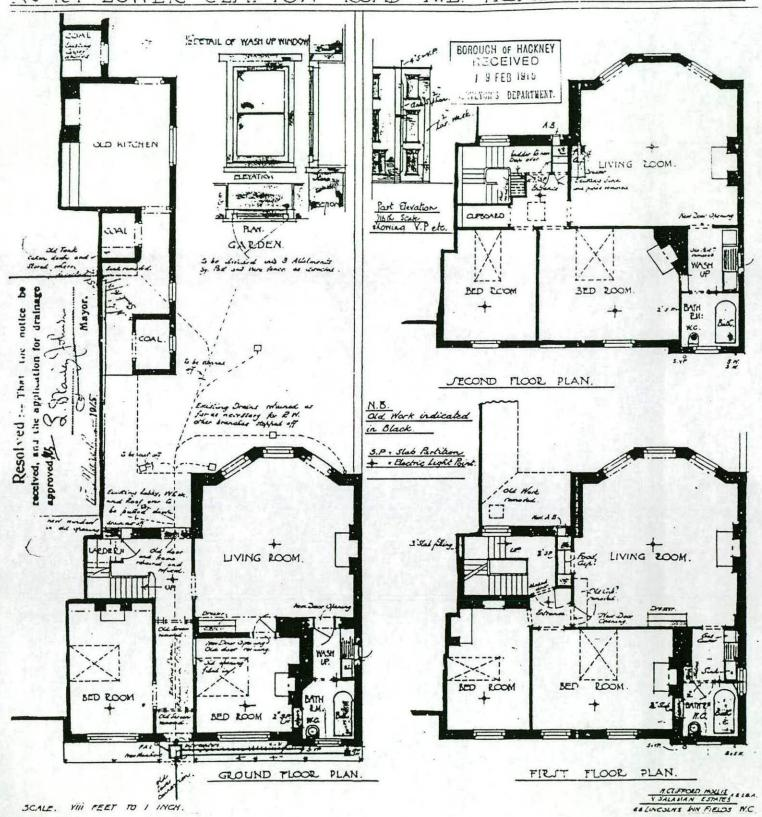
Figure 21. Floor plans showing proposed alterations, 1915
