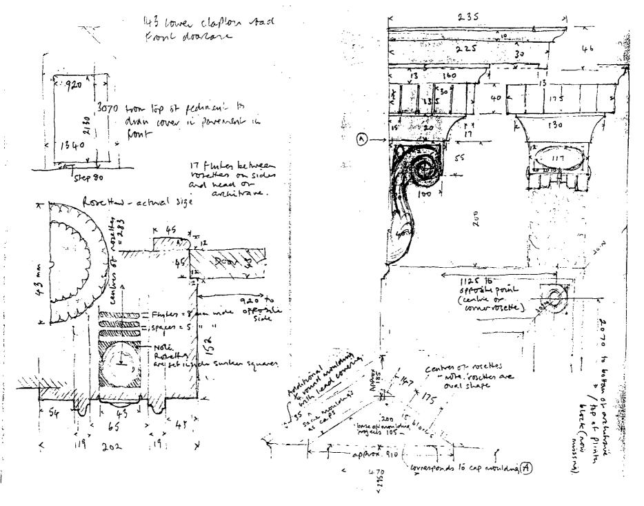
Figure 18. Measured sketches of doorcase details
