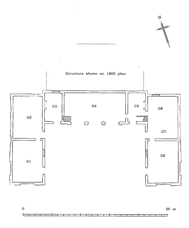
10. Reconstructed first floor plan of the stable block as built c1804, scale 1:200.
