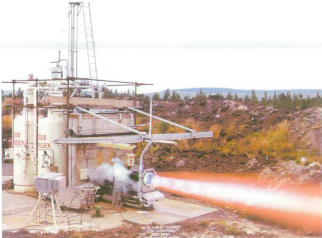
Figure 17 A single firing of the Liquid Hydrogen- Liquid Oxygen Thrust Chamber Facility at Spadeadam was made in 1969 © Rolls-Royce plc
