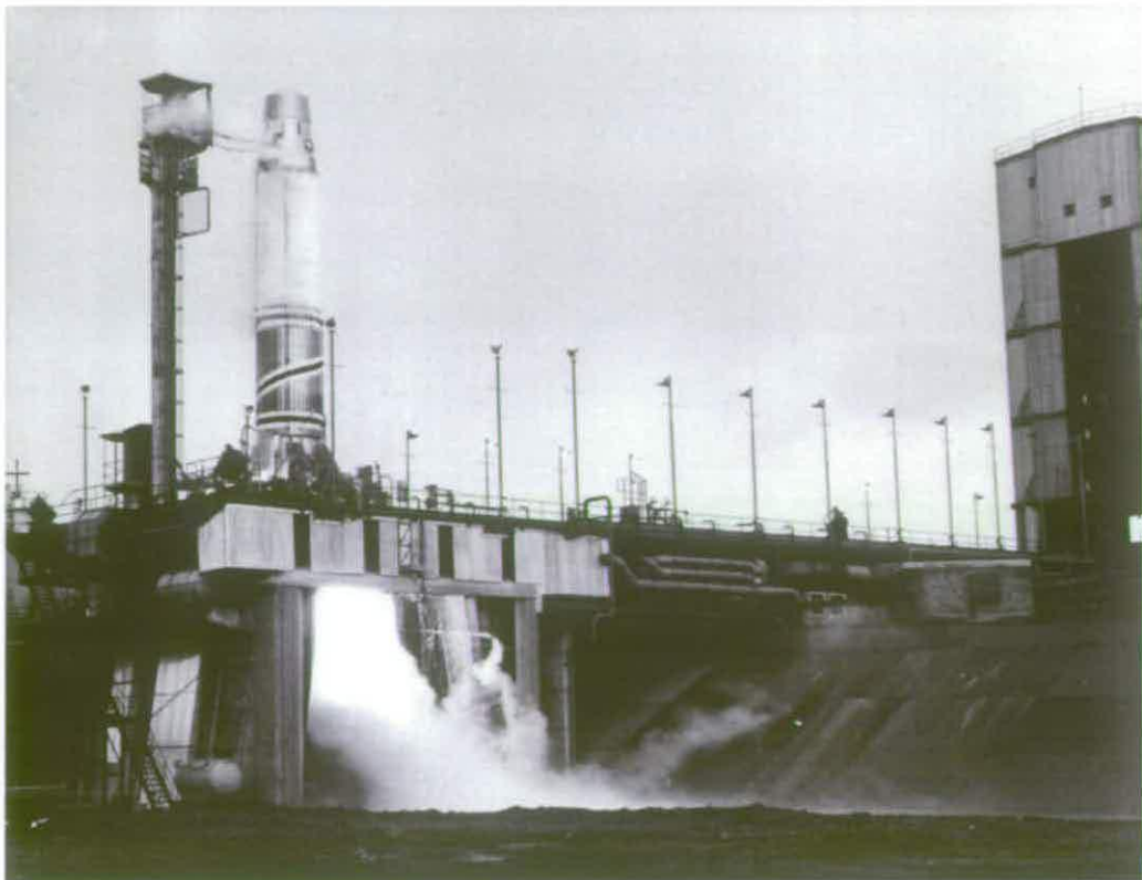
Figure 241 Full rocket firing at Missile Test Stand C3, Greymare Hill © Rolls-Royce plc
