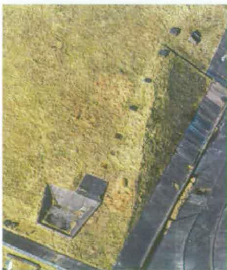
Figure 147 To the west of Test Stand A1 a line of concrete stanchions supported a pipeline leading down to the emergency LOX Dump Tank © English Heritage NMR (17818/17)
