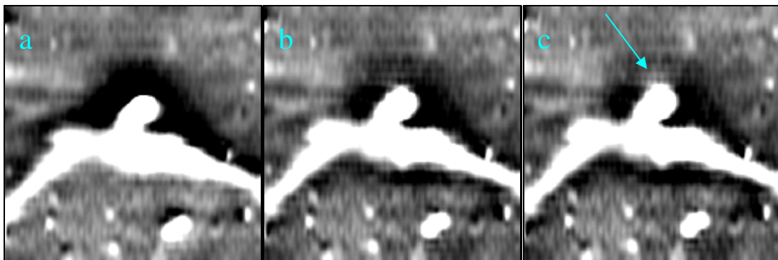
Plate 2, the anomaly at [6]: a) as it appears in the survey; b) after reduction to pole using the present day geomagnetic field direction at Shapwick; c) after reduction to pole using the field direction prevailing in 224 AD [dec = 2.1°; inc = 57.2°] – note the indicated distortion [grey instead of black] to the north of the anomaly.
