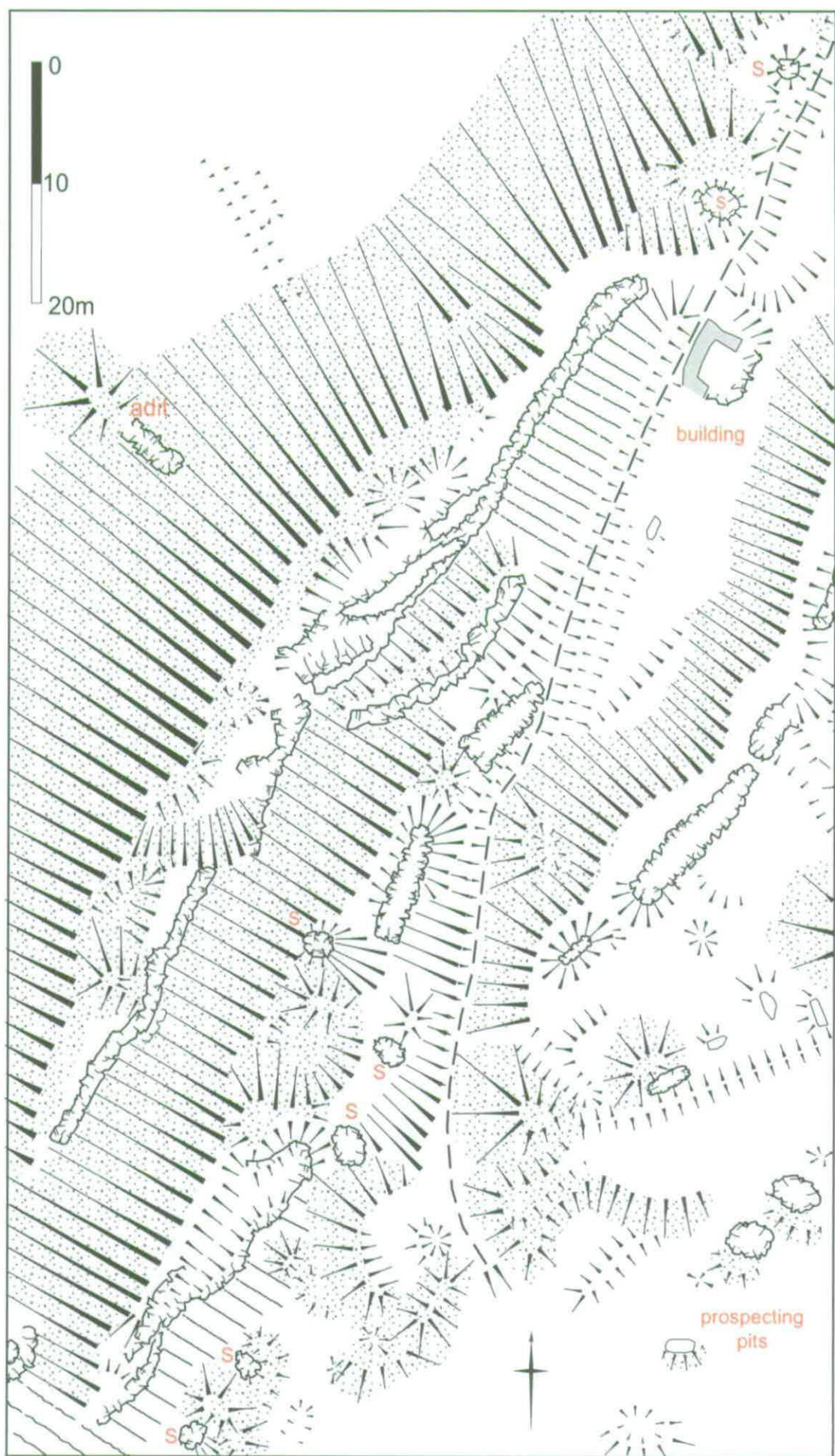
Figure 8. 1:500 scale earthwork plan showing gunnises at the northern end of lode A and lode B (area B on Fig. 4).
