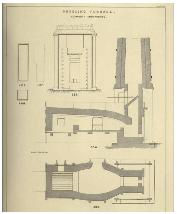
Figure 3. Mid-19th century puddling furnace (Truran 1862, Plate 49)
