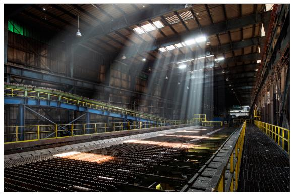
Figure 10. Cooling bed in the rolling mill of Sheerness Steel Works, prior to demolition in 2017 (DP181849, Historic England Archive).
