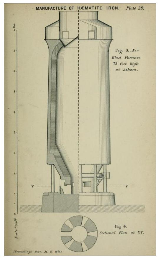
Figure 4. Typical late 19<sup>th</sup> century blast furnace, with a charging gallery, bell hopper and five tuyere openings above the hearth (Proceedings of the Institute of Mechanical Engineers, 1871).
