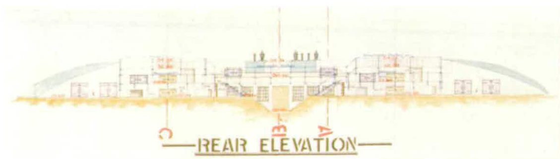
Figure 10 Extract of the 1902 record plan, showing the rear elevation of the 4.7-inch QF gun battery (PRO: WO 78/5139/2; reproduced with the kind permission of the National Archives)
