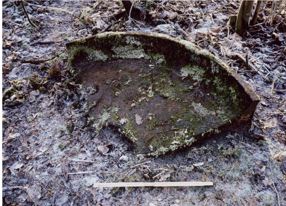
Figure 22. Detail of iron edge- runner fragment outside waterwheel house of early range of incorporating mills. (NMR: AA 012876)
