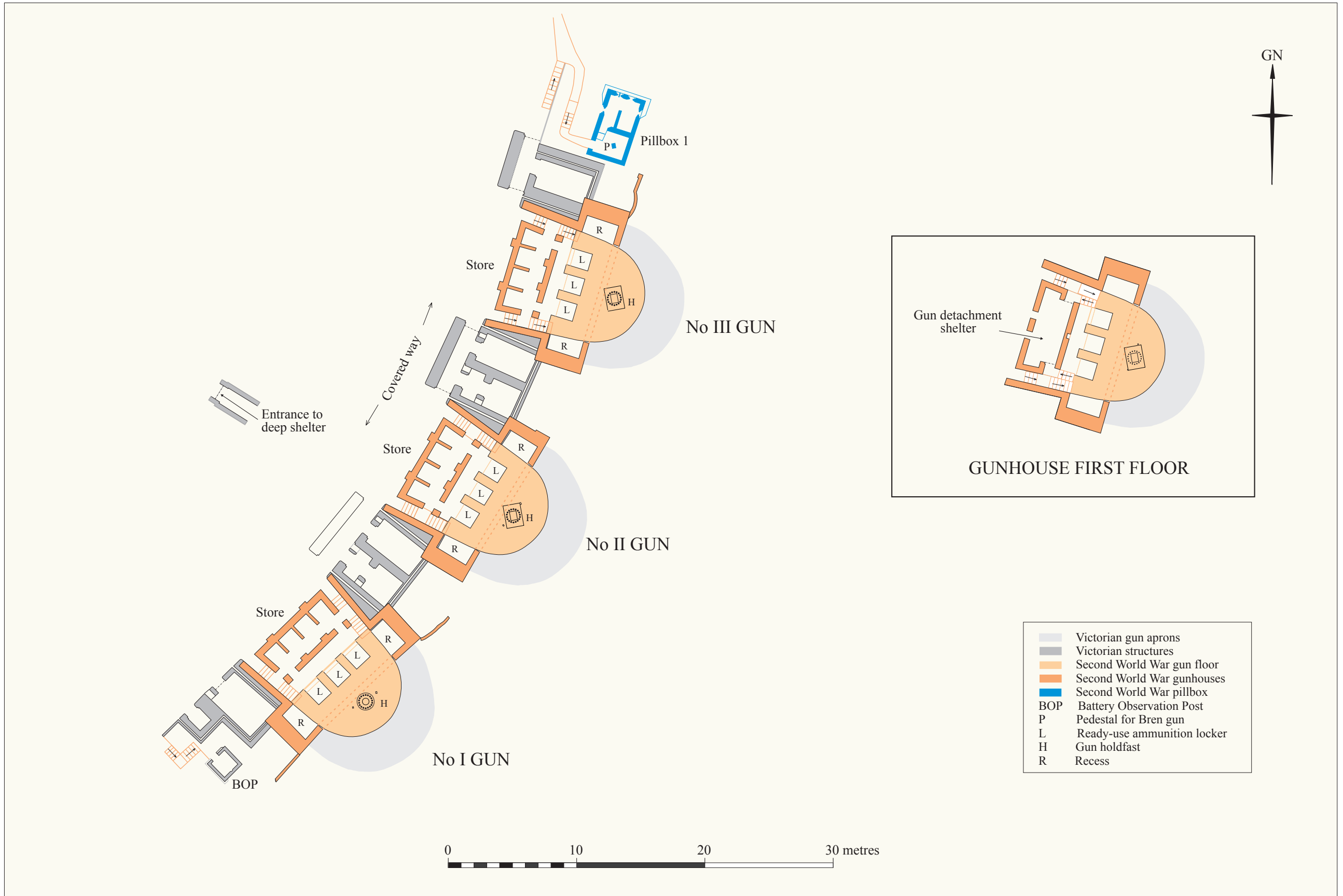
Figure 12 Western Heights Battery: RCHME survey plan of the 'emergency' 6-inch battery of 1940-7
