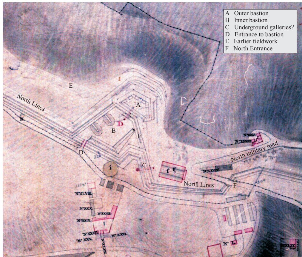
Figure 3 Plan of North Centre Bastion, showing the principal features in 1810. Text in black, excluding Roman numerals, is added by the author (extract of MR1/1349 © The Public Record Office)
