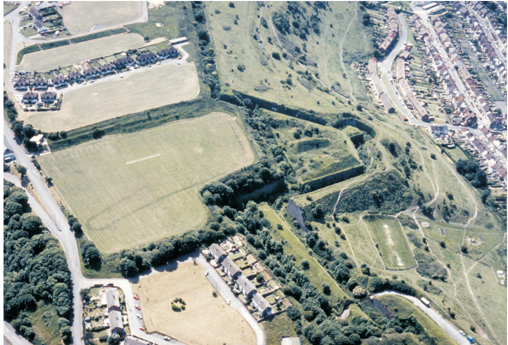
North Centre and Detached Bastions from the air in 1994, showing the prominent northward projection (the right of the photo) in order to flank the slope of Western Heights (©NMR: TR 3140/10, 30th June 1994)
