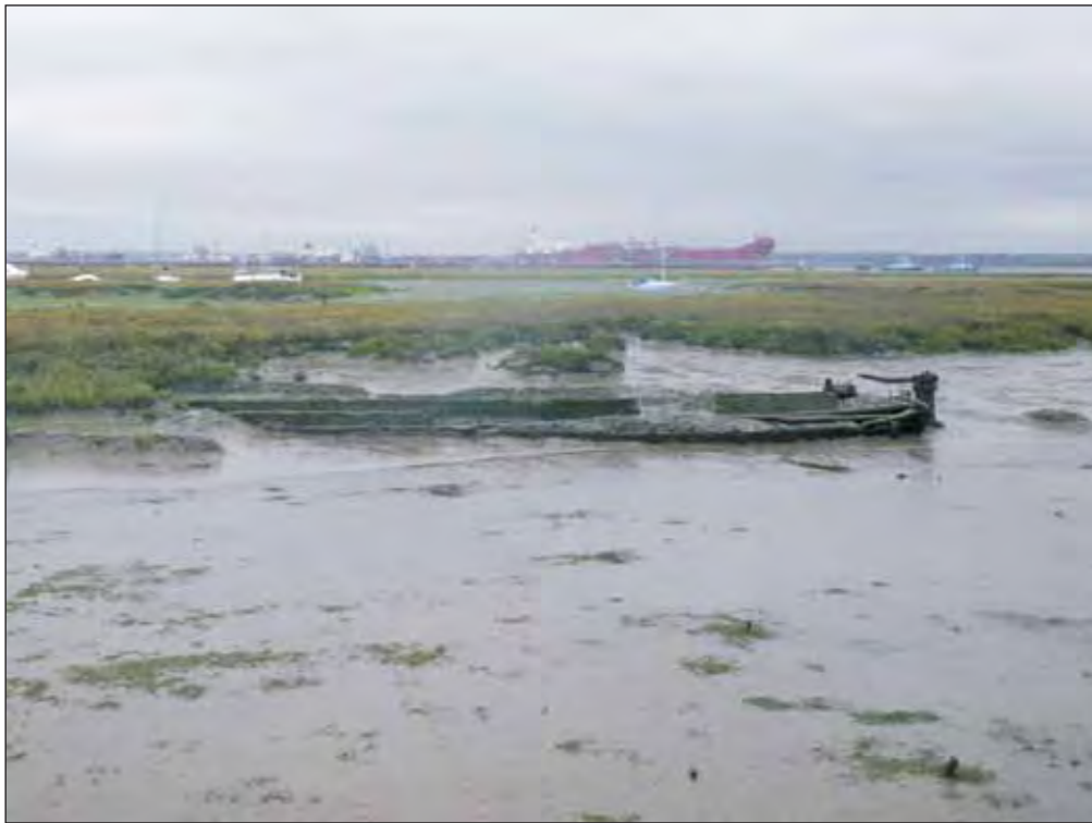
Plate E20: WA5051 . Remains of a wooden barge located in the intertidal area at Ashlett. The vessel is between 10m and 15m long and is in a deteriorated state. There are remains of metal fittings on the interior and the wooden rudder is still intact
