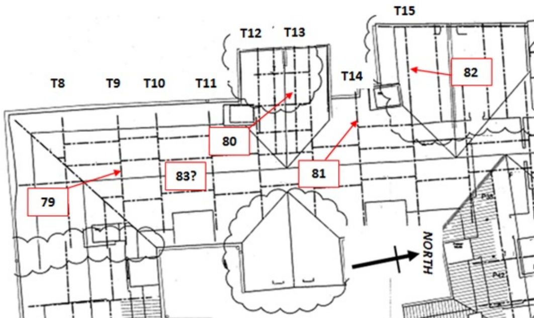
Figure 11: Annotated plan to show locations of sliced samples SYD-H79 – H83 from the ex situ timbers of the West Range roof (after Rodney Melville & Partners)
