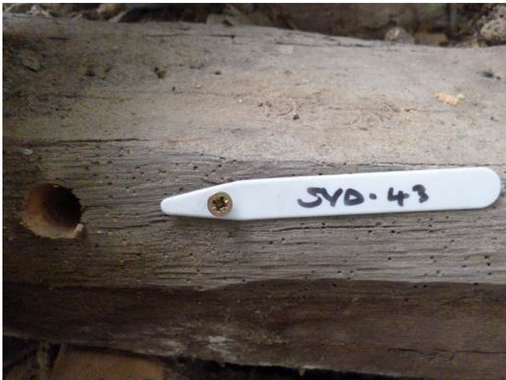
Figure 8a/b: Views to show the labelling of sampled timbers (photographs Robert Howard)
