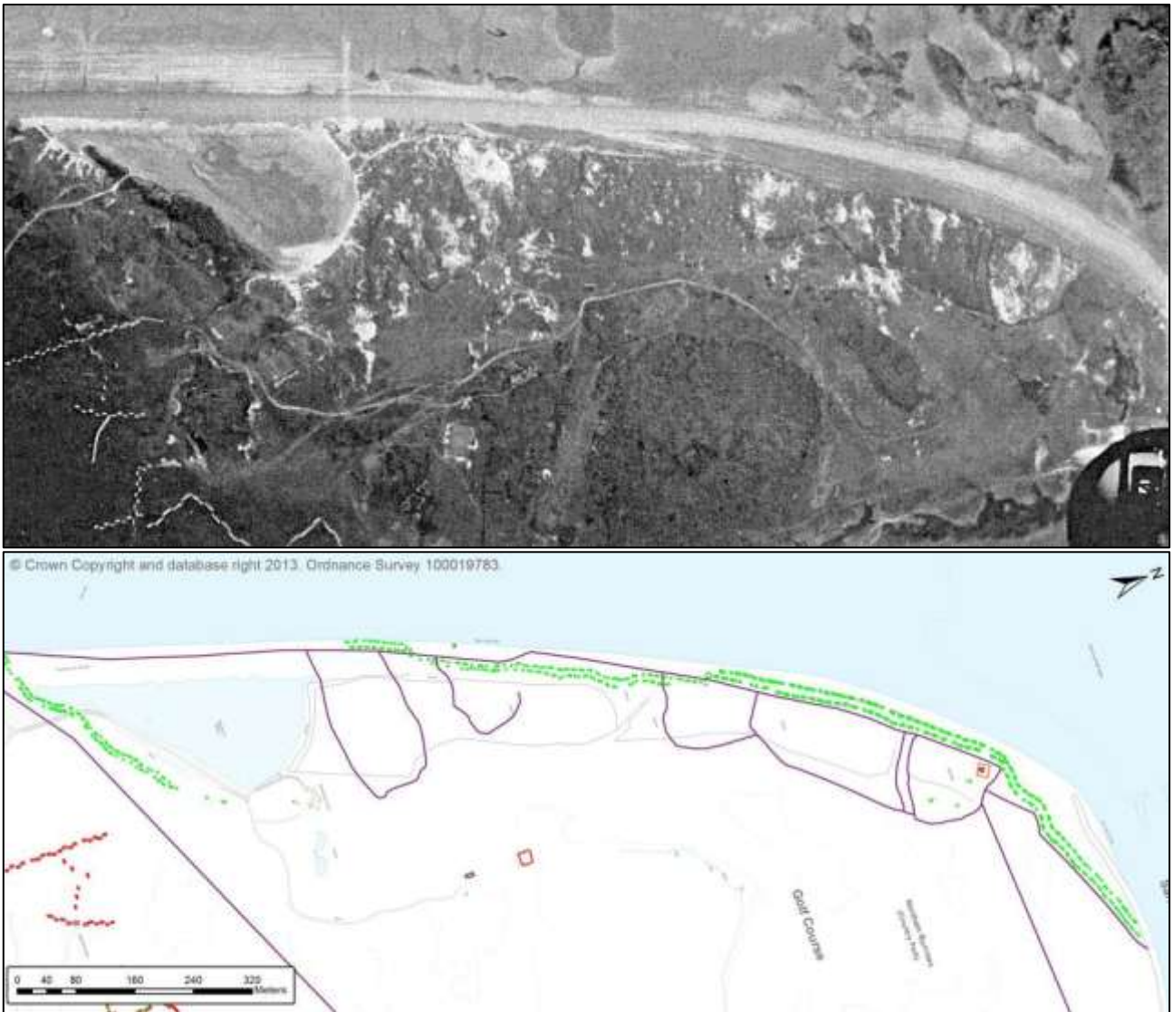
Figure 19. Top: Anti-glider obstructions on Northam Burrows are visible to the left of the image. Barbed wire obstructions defining linear defences and small enclosures are visible as a dark line. Photograph: RAF/S171 15 01-JUN-1941. English Heritage (RAF Photography). Bottom: NMP Transcription, Minefields are green, barbed-wire structures are purple. NMP mapping © English Heritage.
