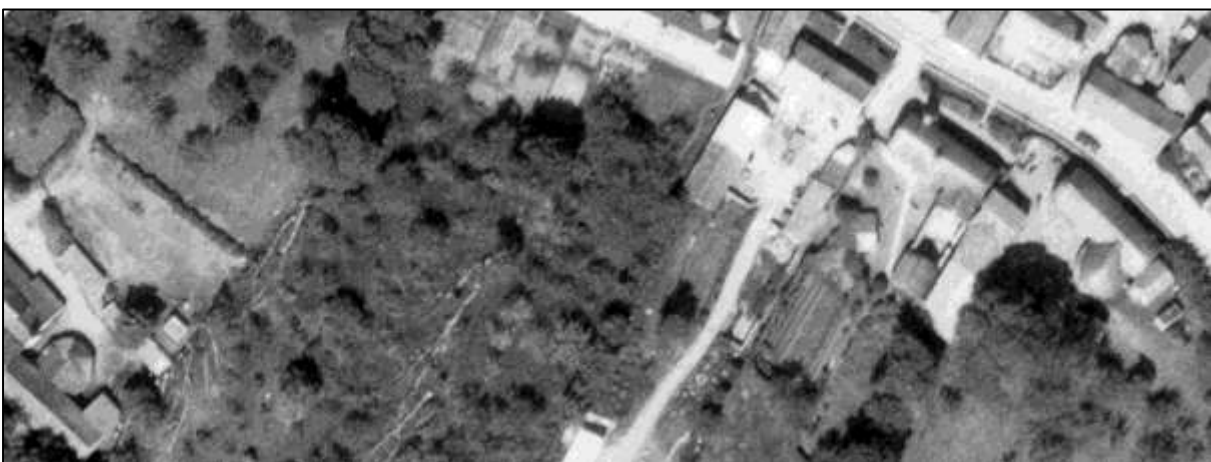
Figure 130. Horse engine houses in Croyde in the 1950s (one bottom left and two far right). These circular appendages were built onto barns to house a horse whim for threshing. This small concentration is visible and apparently still in use, or at least roofed, in 1953, but none are now extant. NMR RAF/58/1133 F22 0001 28-MAY-1953. English Heritage (RAF Photography).
