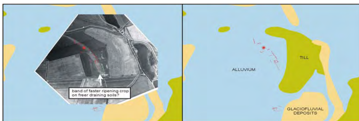
Figure 2 - Left, aerial photograph (HCC HL19 25-JUN-1989) showing crop marks within a band of riper crop and presumed freer draining soil. Right this band is not differentiated in the BGS mapping of the superficial geology.
