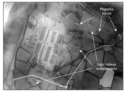
Figure 10-4 The National Shell Filling Factory (No. 23) at Chittening, north of Avonmouth. The original layout can clearly be seen with the light railway embankments. Only two buildings remain unchanged today part of what is now a modern industrial estate.
