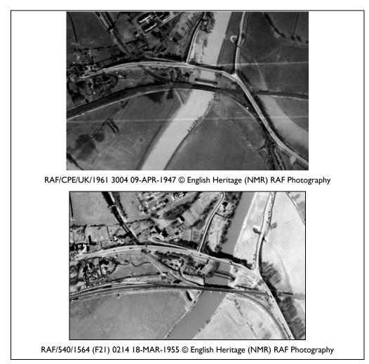
Figure 10-2 Aerial photograph of Over depicting the Telford road bridge (top), gas pipeline (middle) and Brunel's railway bridge (bottom) over the River Severn. Note the realignment of the railway bridge in the 1955 photograph.
