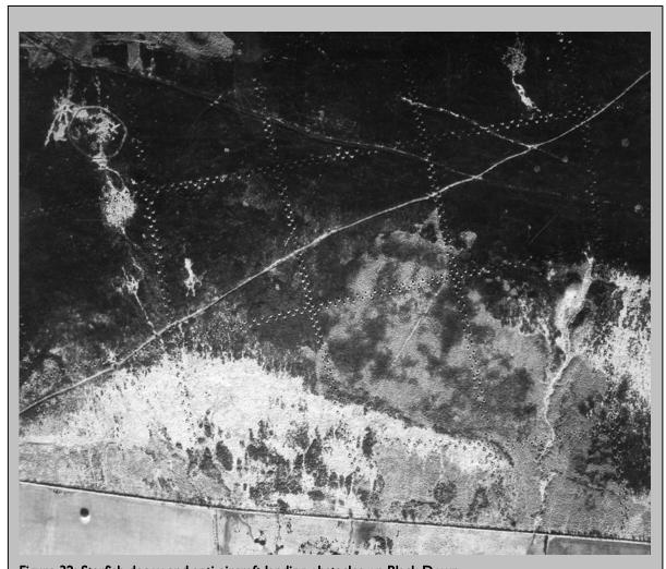
Figure 32: Starfish decoy and anti-aircraft landing obstacles on Black Down RAF 3G/TUD/UK/15/21 PART IV 5356 13-JAN-1946 English Heritage (NMR) RAF Photography
