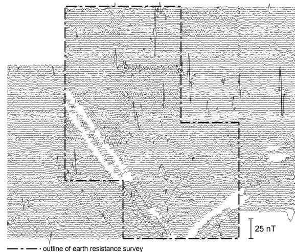
i) Traceplot of magnetometer data after drift correction and range truncation
