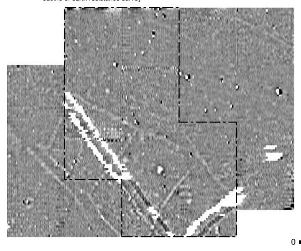
ii) Linear greyscale plot of magnetometer data after drift correction and range truncation
