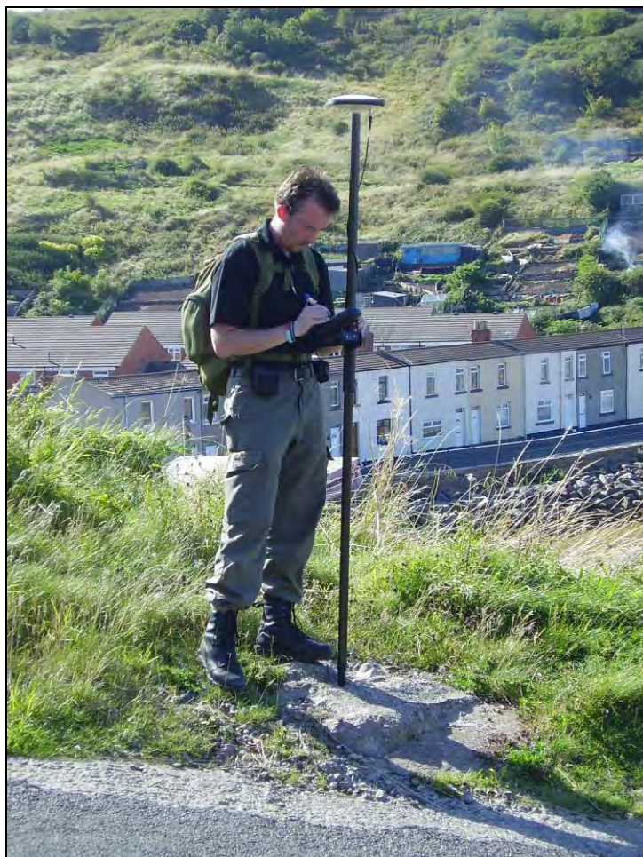
Fig 4.1 Utilising the Magellan CX mapping grade GPS with external antenna for post processing, at Skinnigrove.
