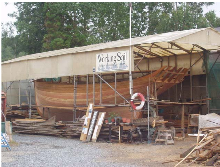
Fig 16 Construction of an Isles of Scilly Pilot Cutter at Gweek boat yard, Cornwall, in 2007 (© Bill Booth and licensed for reuse under this Creative Commons Licence .)
